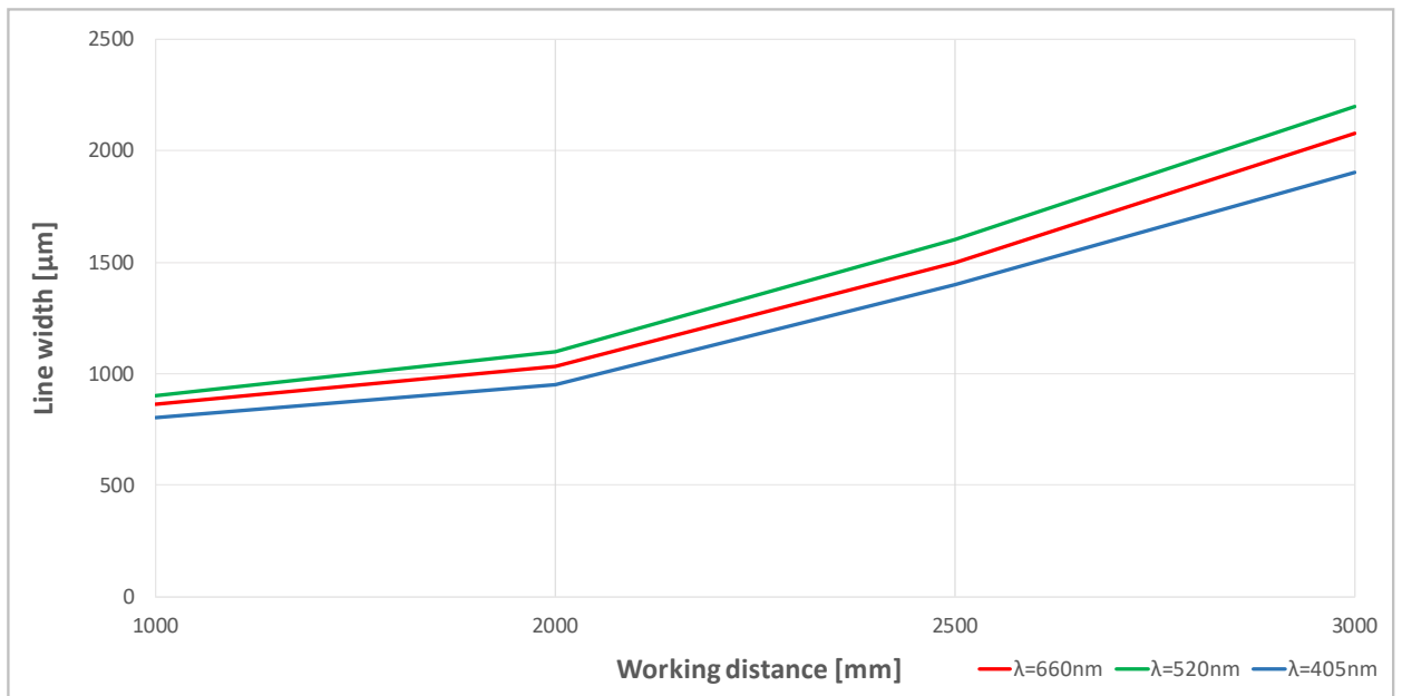
Fig. 2: Typical line width of a collimated line laser module
